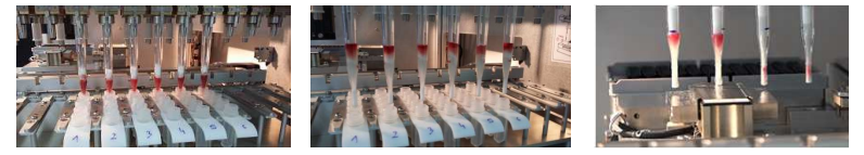
Figure 4. Run Preparation : • Ready-to-use strip concept with embedded reagents • 2min hand-on-time to load & fill strips with 1mL positive BC • Load Vitek®MS target slide & CHCA, FA, E.Coli calibrant tubes • Up to 12 BC could be extracted simultaneously by the instrument. • Load Rack in the instrument and Start
