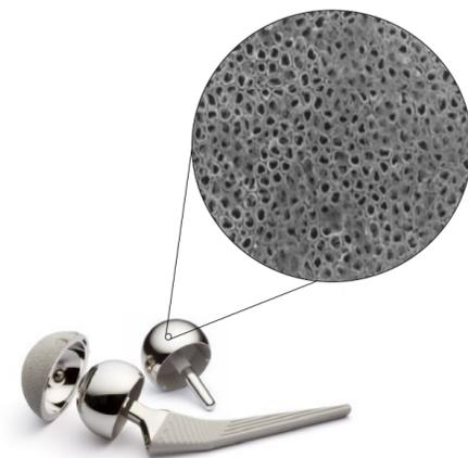
**Figure 1.** Nanoscale micrograph of FT-NT layers on Ti6Al4V alloy.
