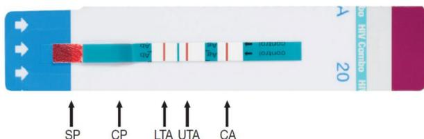
Figure 1 Test strip with sample pad (SP), conjugate pad (CP), lower test area (LTA) for HIV antibody, upper test area (UTA) for HIV-1 p24 antigen, and control area (CA) indicated.
