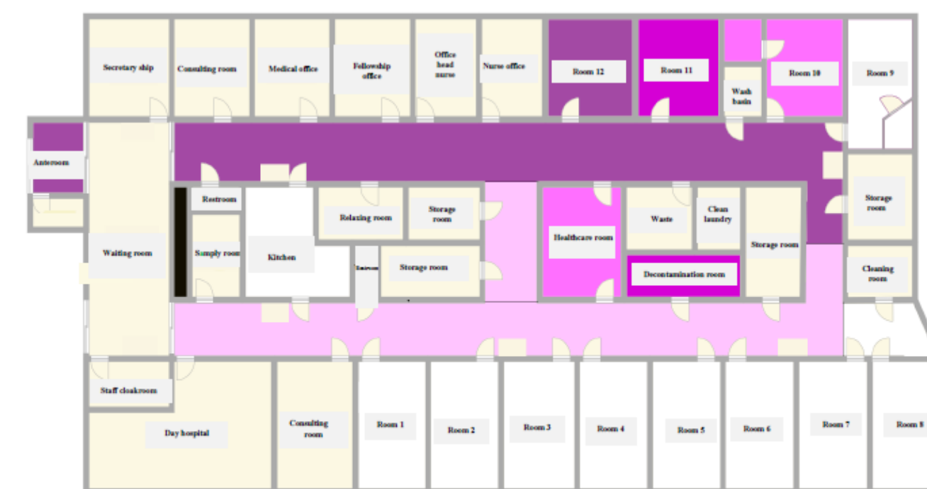
Fungal contamination of the air in the onco-hematology unit during the study period 3: the more purple areas correspond to the most contaminated places
